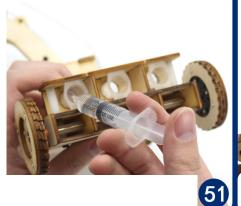
Like in this photo - there is no air inside the tubes, only water. This is important.
