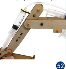
After you fill the tube with water, add back in the plunger.
