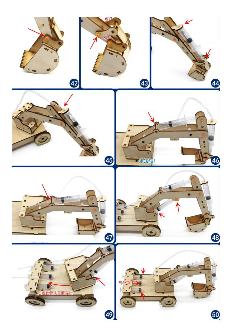
At this point, you need to add water to the tubes. Hold the vehicle at an angle so you can add water all the way down the tube with NO AIR inside.
