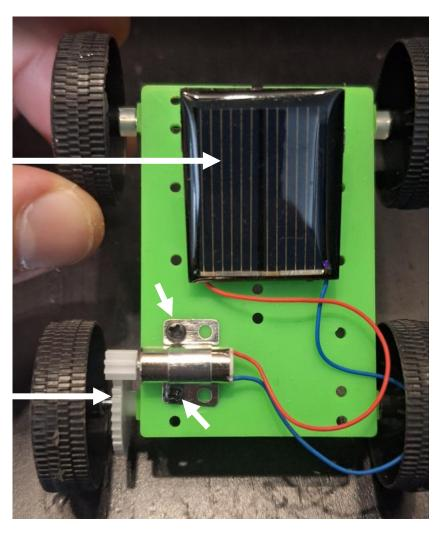
Make sure to install the motor mount in these exact holes. Use the two small screws that were provided.
