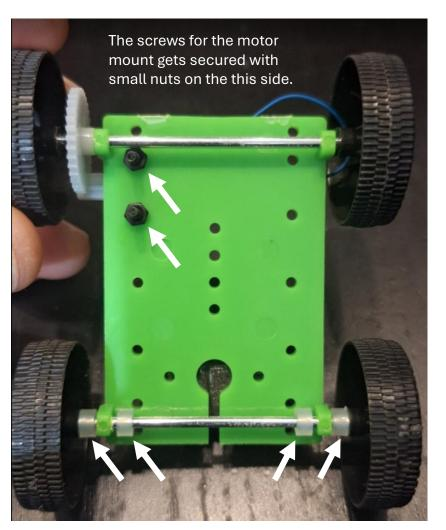
Use the small plastic washers to ensure the axle doesn't slip from side to side.
